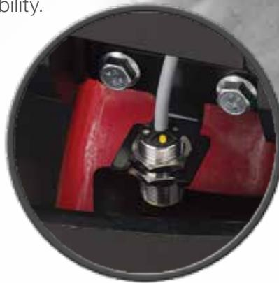
*Smart Slow Down™ Sensor automatically detects significant turns and adjusts truck speed accordingly.*
